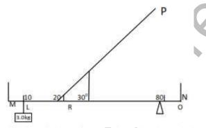
50. In fig. 2; above, MN is a light uniform metre rule pivoted at 0, the 80cm mark. A load of mass 3.0kg is suspended on the, rule at L, the 1.0cm mark. If the rule is kept in equilibrium by a string p, fixed at p and attached to the rule at R, the 20cm mark, then the tension T in the string is A. 25N
